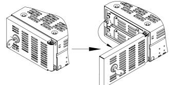
5. Remove the screw with the drive unit intended to replace in the left side.
