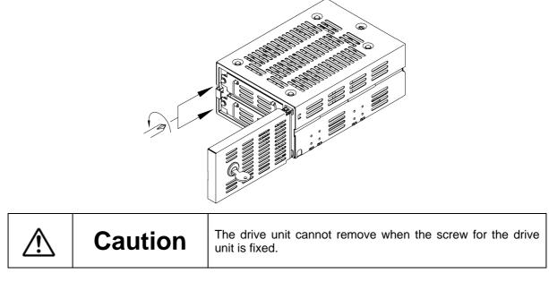
5. Carefully pull out the failed drive unit from the Mirror Drive.
