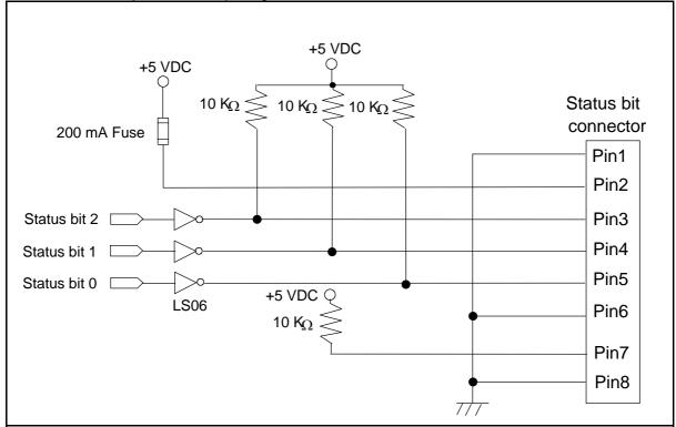
Status output signal uses LS06 (open corrector). Each output has a 10 K pull-up resistor.
