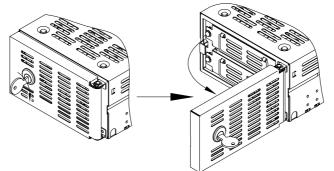
5. Remove the screw with the drive unit intended to replace in the left side.
