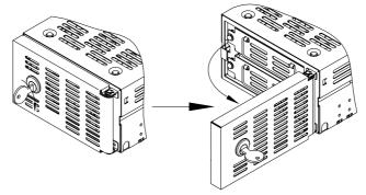
4. Remove the screw with the drive unit intended to replace in the left side.
