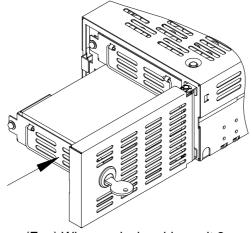
(E.g.) When replacing drive unit 2.
