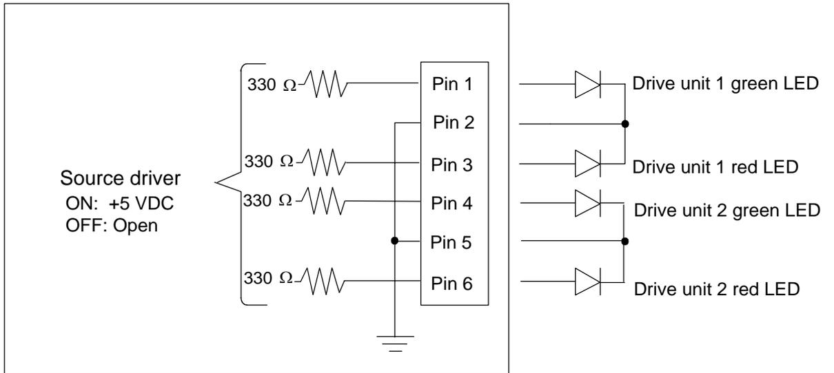
External LED output signal electrical specifications. (The signal pins 1, 3, 4, 6)
