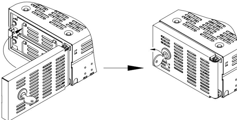
11. Mount the **Mirror Drive** in the host computer and firmly connect the IDE (ATA) cable and 4-pin internal power cable.
