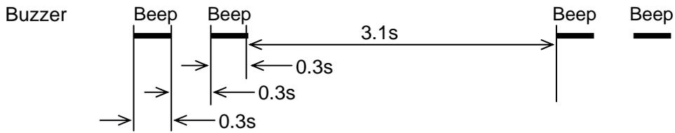
System stopped (Both drive units have failed)
