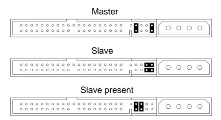
If the slave drive unit is not correctly recognized when set as master, use this setting.
