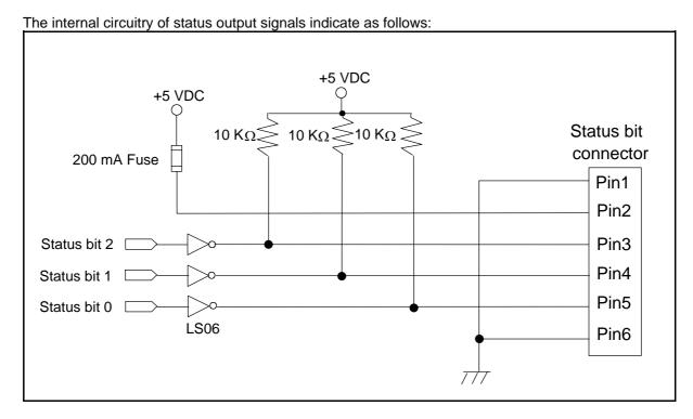
Status output signal uses LS06 (open corrector). Each output has a 10 K pull-up resistor.
