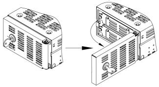
5. Remove the screw with the drive unit intended to replace in the left side.
