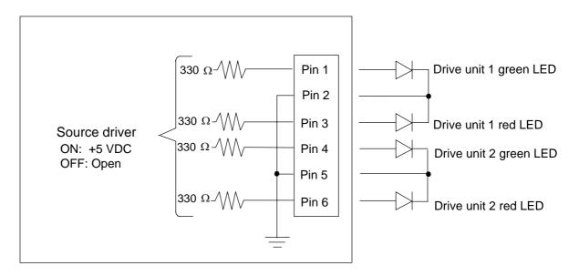
External LED output signal electrical specifications. (The signal pins 1, 3, 4, 6)
