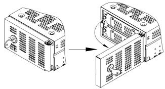
4. Remove the screw with the drive unit intended to replace in the left side.
