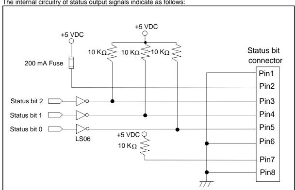
The internal circuitry of status output signals indicate as follows:
