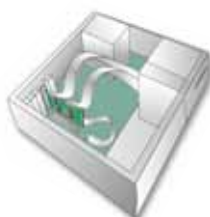
Mirror Card Put into the PCI Slot to realize hardware mirror.
