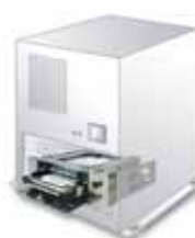
Mirror Drive Just fit in 5.25" Open Bay with hot swap capability.
